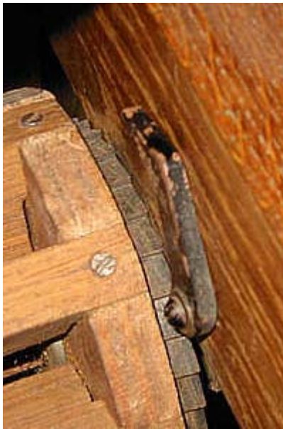
System of blocking of the front roller. Sight of the bobbin and the fixed cog on the side of the roller
