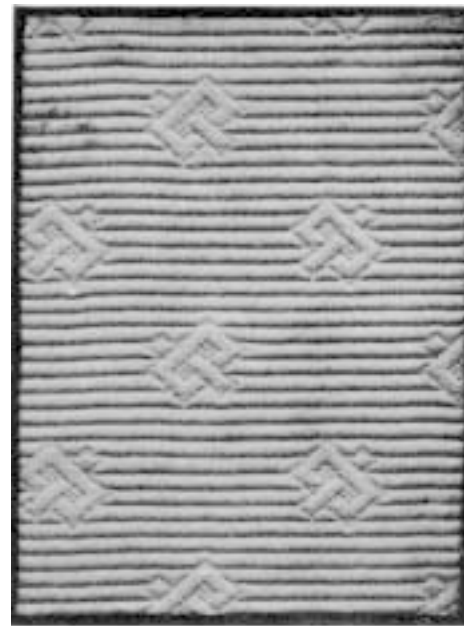
FIG. 605.—Piqué fabric with "toilet" or "quilted" figuring.
