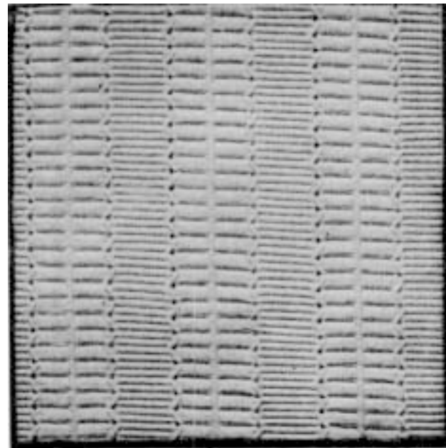
FIG. 609.—Piqué fabric with net leno stripes.
