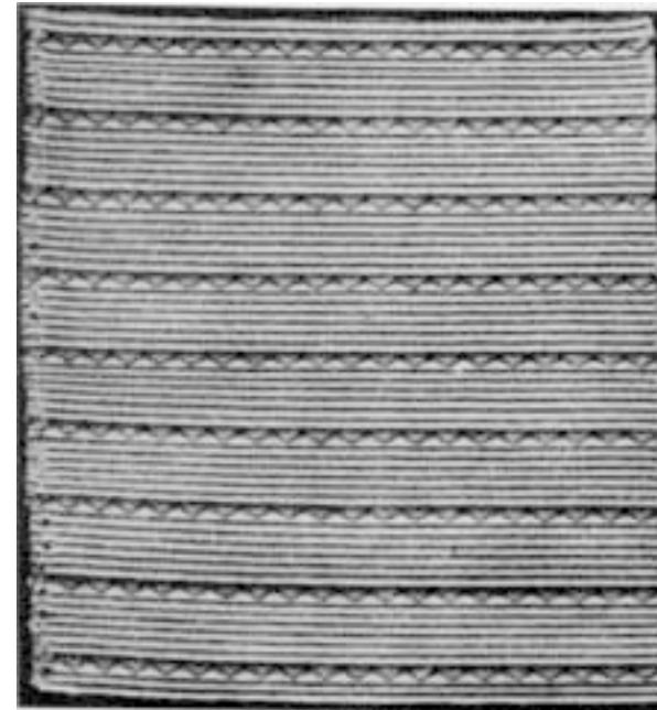
FIG. 600.—Piqué fabric embellished with extra picks of coloured weft.
