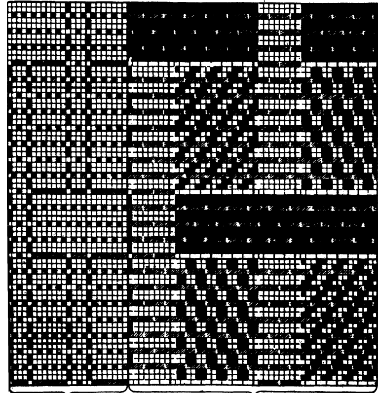
FIG. 615.—Applied design for matelasse fabric with pattern as in block design, Fig. 614.
