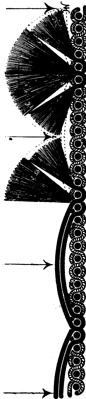
Fig. 381.—Graphic diagram of the transverse section of corduroy fabric, from design Fig. 380, showing certain picks of weft both entire, and also after being severed by the fustian knife to form tufts of pile.
