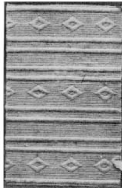
FIG. 606.—Piqué fabric with "toilet" or "quilted" figuring and variegated ribs or welts and of which Fig. 607. is the applied design.
