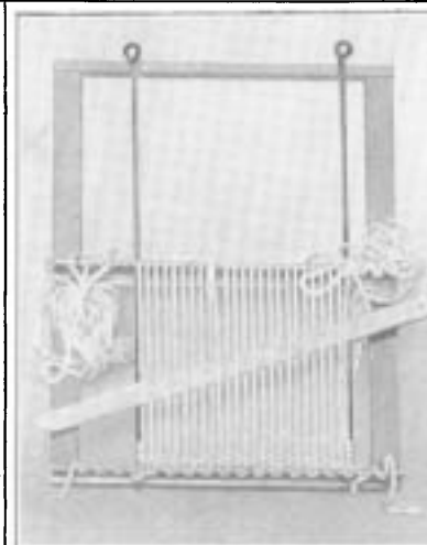
The Todd Loom No. 2 adjusted for 6-inch square
